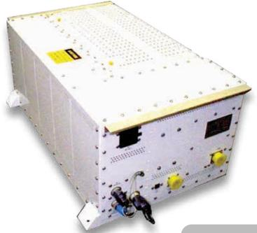
X-Band coupled cavity travelling wave tube transmitter with solid state pre-amplifier. Features a series of resonant high voltage power supply with dual depressed collector stages.
